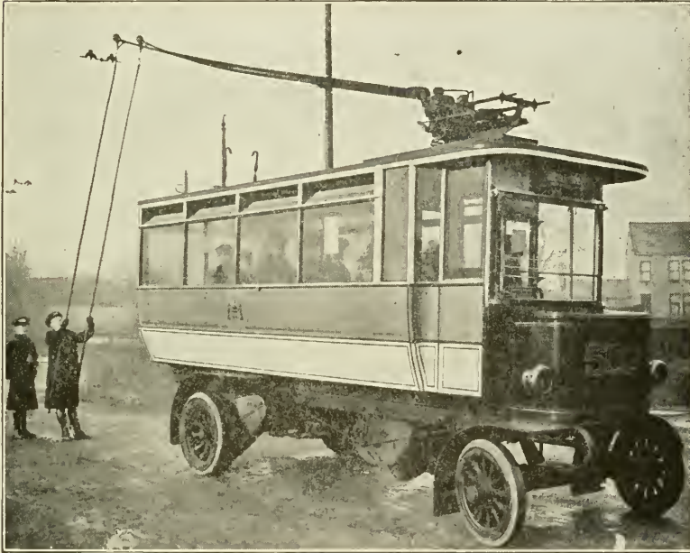
Fig. 16. Leeds Trackless Trolley Car. Guard Shifting Trolleys Courtesy of Southern Electrician
